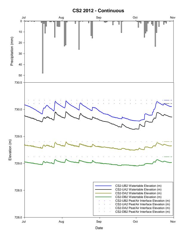
Figure 9. Water table elevation (m), peat/air interface elevation (m) and daily precipitation (mm) for CS2 in 2012, Porcupine Hills, Manitoba (Steeprock Operating Area).
