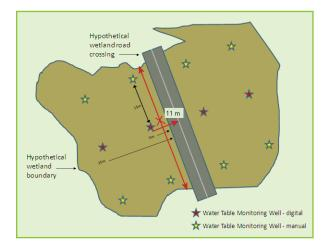
Figure 1. Layout of sampling design showing placement and location of digital and manual water table monitoring wells. Courtesy of Ducks Unlimited Canada.
