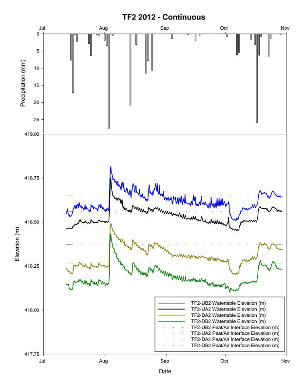
Figure 18. Water table elevation (m), peat/air interface elevation (m) and daily precipitation (mm) for TF2 in 2012, Pasquia Hills, Saskatchewan.
