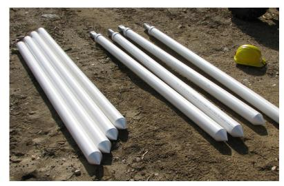
Figure 4. Monitoring wells were made of perforated PVC plastic pipe with conical shaped bottoms. A stretchable fabric sock installed around the pipe (not shown in picture) kept sediment and debris from entering the well through the perforations. Wells had either a removable cap on top to allow for manual water level measurements and sampling (left) or a digital water level recorder as the cap (right).
