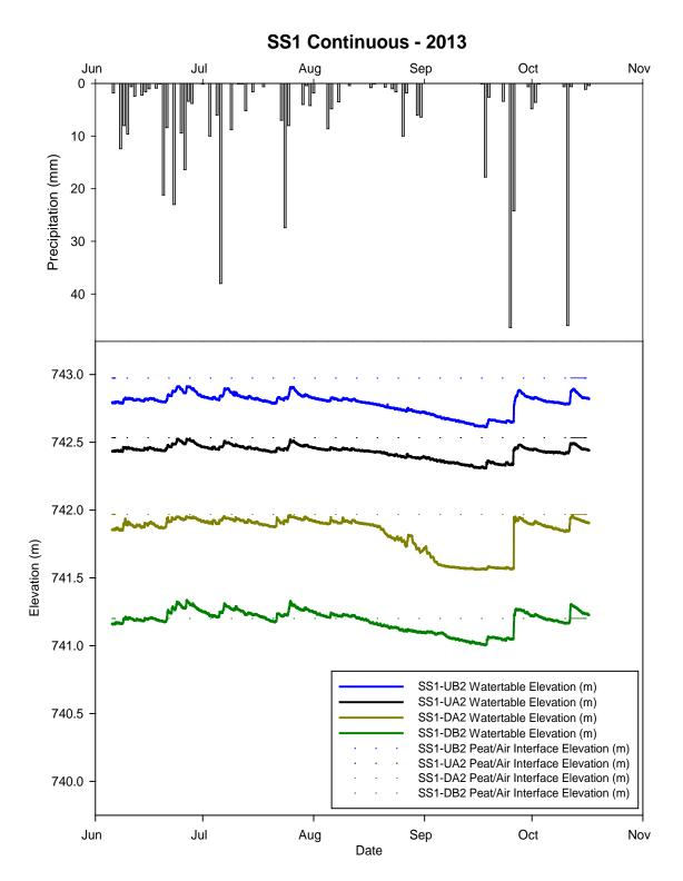
Figure 4. Water table elevation (m), peat/air interface elevation (m) and daily precipitation (mm) for SS1 in 2013, Porcupine Hills, Manitoba (Steeprock Operating Area).
