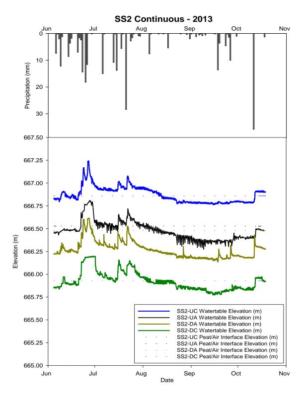
Figure 16. Water table elevation (m), peat/air interface elevation (m) and daily precipitation (mm) for SS2 in 2013, Ducks Mountains, Manitoba (Upper Dam Operating Area).
