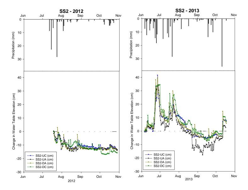
Figure 17. Net change in water table elevation after initial reading and daily precipitation in 2012 and 2013 at site SS2 in Duck Mountains, Manitoba (Upper Dam Operating Area).
