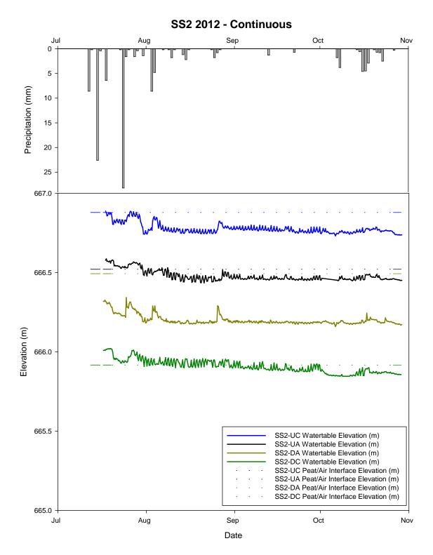
Figure 15. Water table elevation (m), peat/air interface elevation (m) and daily precipitation (mm) for SS2 in 2012, Duck Mountians, Manitoba (Upper Dam Operating Area).
