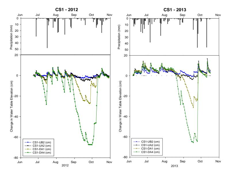
Figure 8. Net change in water table elevation after initial reading and daily precipitation in 2012 and 2013 at site CS1 in Porcupine Hills, Manitoba (Steeprock Operating Area).
