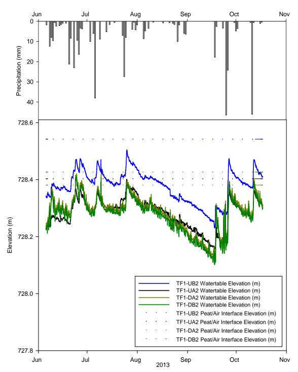
Figure 13. Water table elevation (m), peat/air interface elevation (m) and daily precipitation (mm) for TF1 in 2013, Porcupine Hills, Manitoba (Steeprock Operating Area).
