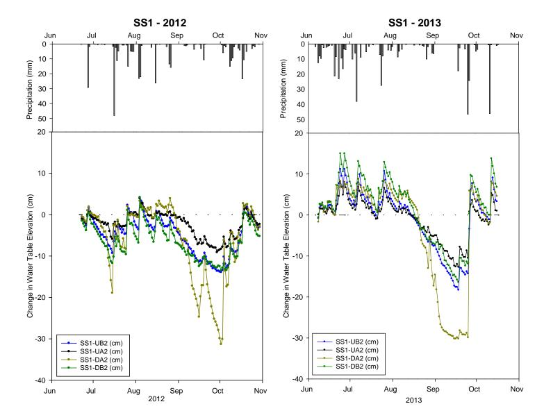
Figure 5.Net change in water table elevation after initial reading and daily precipitation in 2012 and 2013 at site SS1 in<br/>Porcupine Hills, Manitoba (Steeprock Operating Area).
