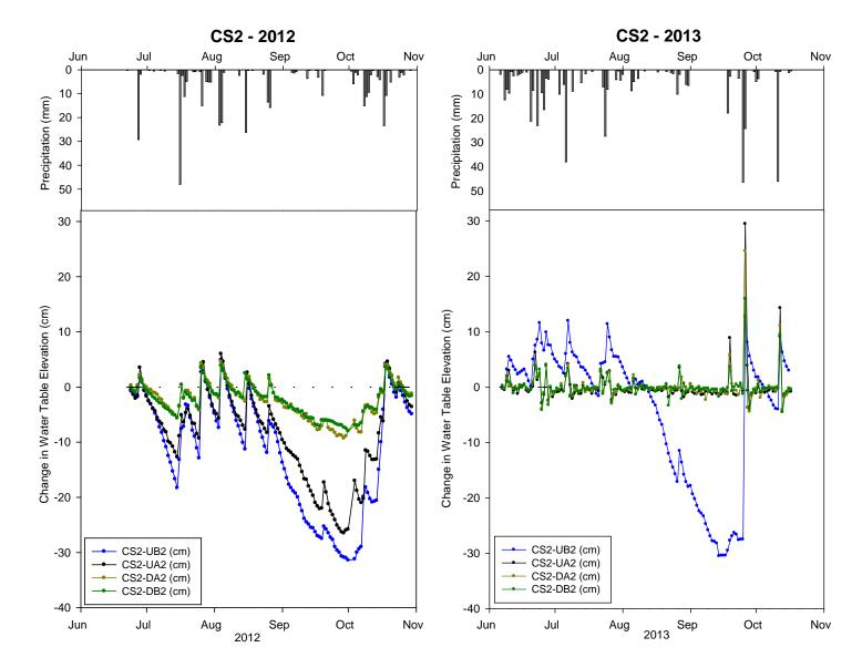
Figure 11. Net change in water table elevation after initial reading and daily precipitation in 2012 and 2013 at site CS2 in Porcupine Hills, Manitoba (Steeprock Operating Area).
