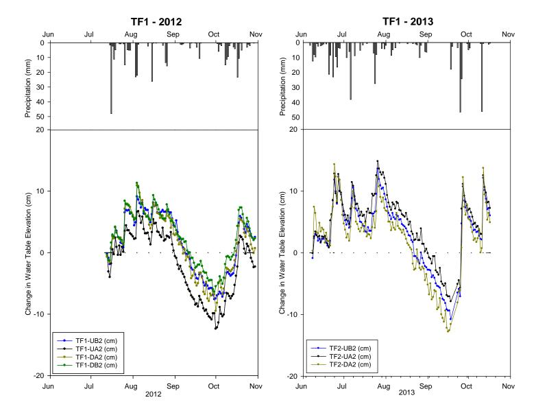
Figure 14. Net change in water table elevation after initial reading and daily precipitation in 2012 and 2013 at site TF1 in Porcupine Hills, Manitoba (Steeprock Operating Area).
