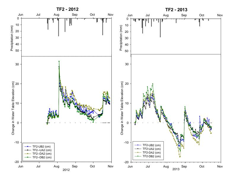
Figure 20. Net change in water table elevation after initial reading and daily precipitation in 2012 and 2013 at site TF2 in Pasquia Hills, Saskatchewan.
