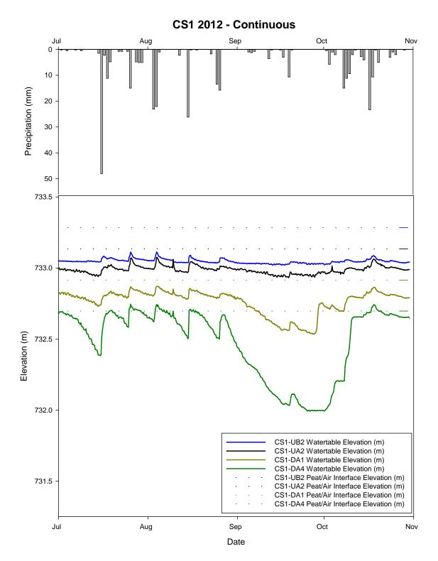
Figure 6. Water table elevation (m), peat/air interface elevation (m) and daily precipitation (mm) for CS1 in 2012, Porcupine Hills, Manitoba (Steeprock Operating Area).
