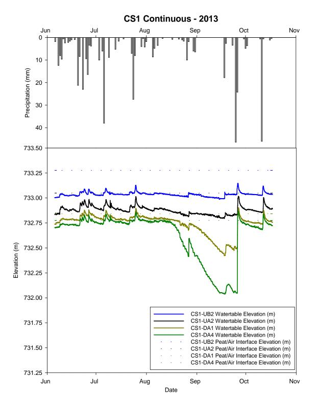
Figure 7. Water table elevation (m), peat/air interface elevation (m) and daily precipitation (mm) for CS1 in 2013, Porcupine Hills, Manitoba (Steeprock Operating Area).
