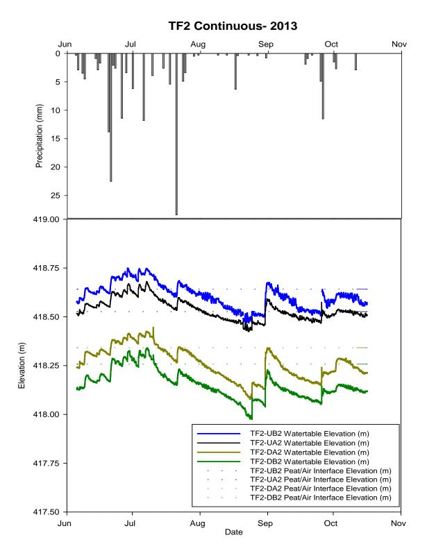
Figure 19. Water table elevation (m), peat/air interface elevation (m) and daily precipitation (mm) for TF2 in 2013, Pasquia Hills, Saskatchewan.
