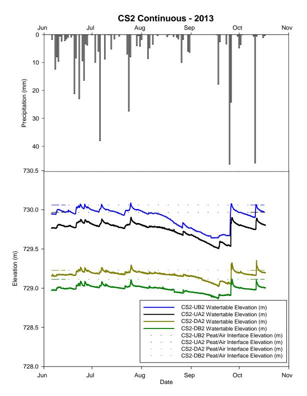
Figure 10. Water table elevation (m), peat/air interface elevation (m) and daily precipitation (mm) for CS2 in 2013, Porcupine Hills, Manitoba (Steeprock Operating Area).
